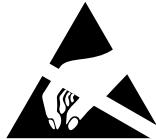
**This product can be damaged by electrostatic discharge (ESD). Handle with appropriate precautions.**
